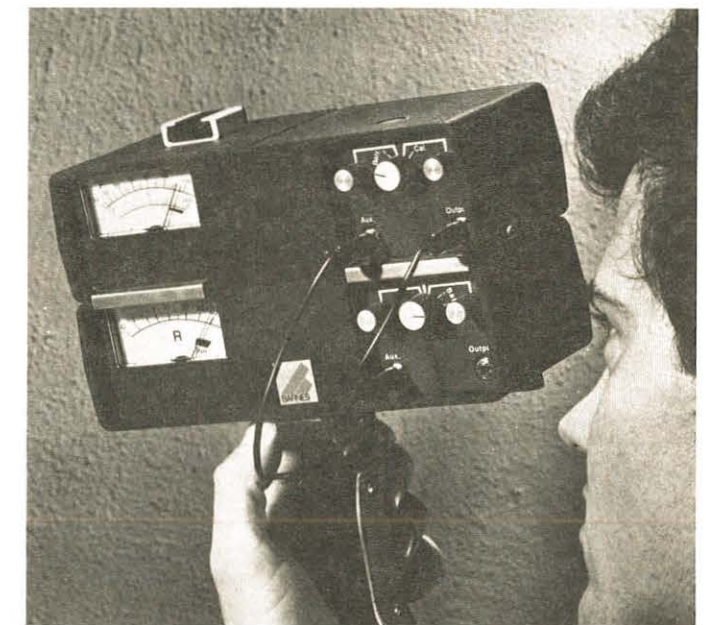
New R-value meter from Barnes Engineering Co.
