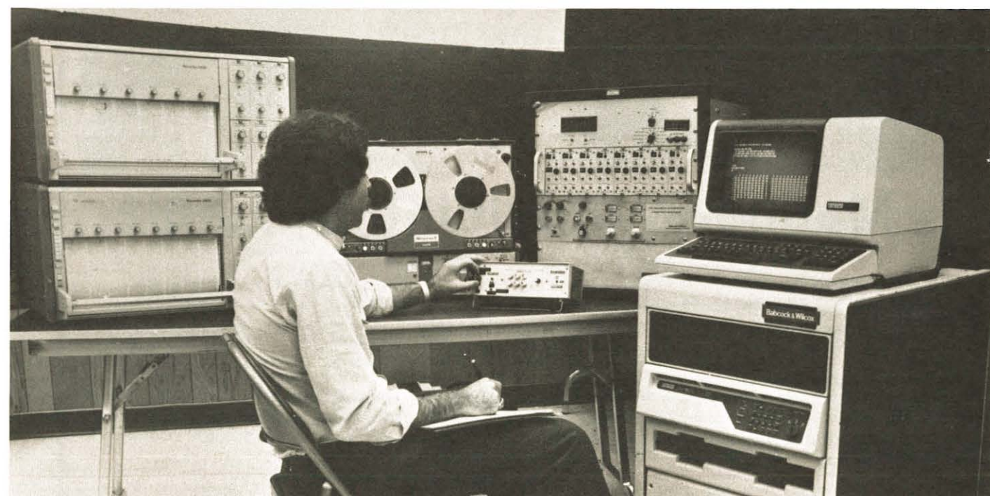
Nuclear Inspection System — Babcock & Wilcox, Lynchburg, VA, data acquisition equipment records profilometry probe measurements on magnetic tape and strip charts. Data analysis equipment reduces the information to numeric estimates of strain and then plots tube profiles. This is part of B&W's nuclear inspection system to avert unnecessary tube plugging in nuclear power plants.
