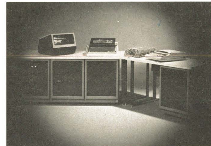
This new Hewlett-Packard Model 3060A Option 100 system tests complex microprocessor circuit boards.
